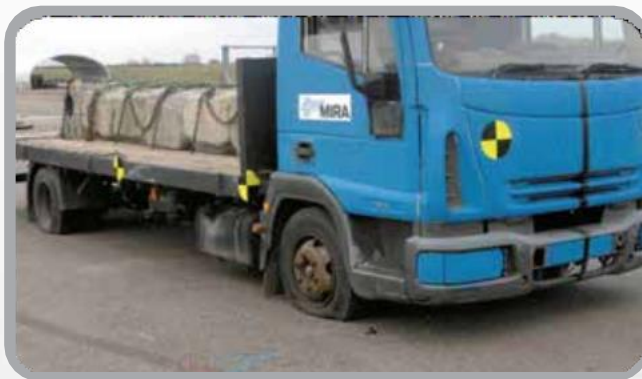
Post Test : All tyres deflated immediately
