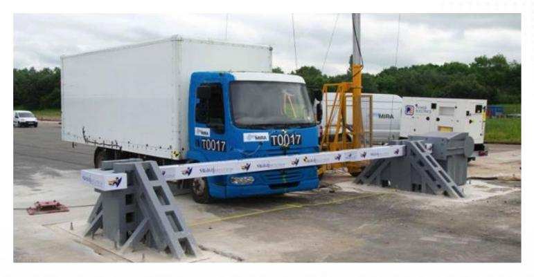
Swaraj Secutech presents India's first indigenously designed and manufactured Crash Rated Boom Barrier. The Barrier has been impact rated in accordance with IWA 14-1:2013 std at Horiba MIRA, U.K. wherein the barrier was hit at 64 km/h by a fully laden 7.2-ton truck.
