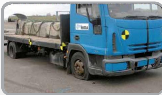
Post Test : All tyres deflated immediately
