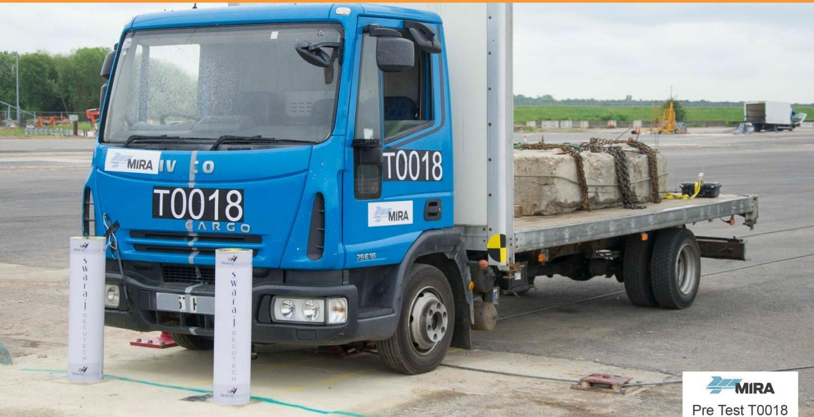
Swaraj Secutech presents India's first indigenously manufactured and physically crash rated bollard. Our bollards have been impact rated by Horiba Mira. U.K. wherein the bollard was hit by a fully laden 7.2-ton truck at 48 km/h and still achieved a penetration of only 0.1m.
